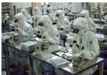
无尘室内全检 (无尘等级: 1000) Full Inspection In A Clean Room
